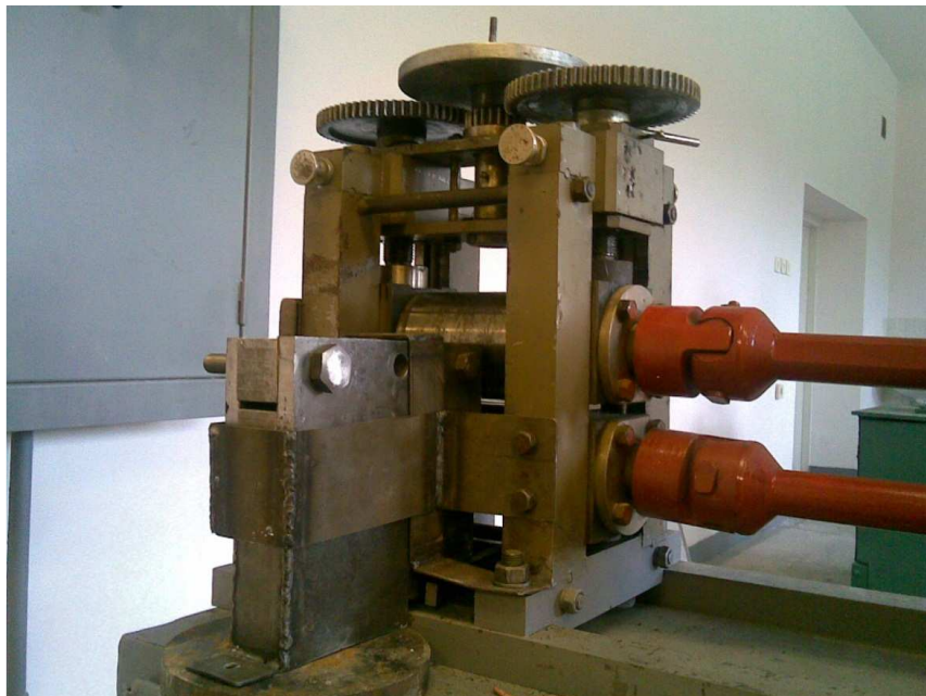
Fig. 2 – Machine for realization of combined process “rolling-pressing”
